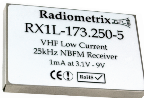
Radiometrix RX1L radio receiver combines 'always-on' convenience with long battery life
