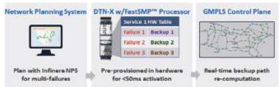
Infinera SMP components, with NPS, FastSMP processor and GMPLS control plain
