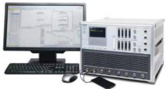
Application-layer demonstration featuring MD8430A LTE simulator uses 10 simultaneous 100 Mb/s data streams to achieve peak throughput
