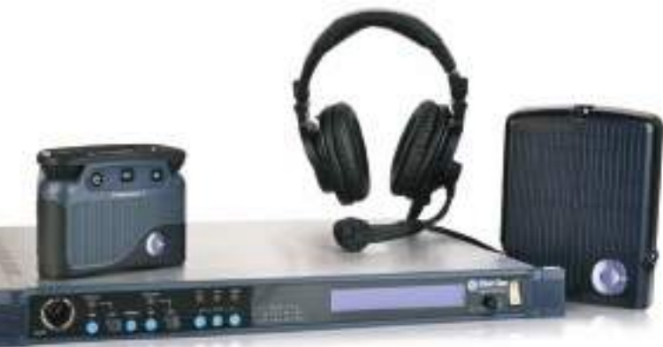
FreeSpeak II systems can co-operate with a mix of 1.9GHz and 2.4GHz belt-packs and antennas
