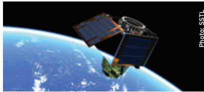
DarkCarb technology demonstration mission flying low-cost MWIR detector, targeted for 2021 launch.
