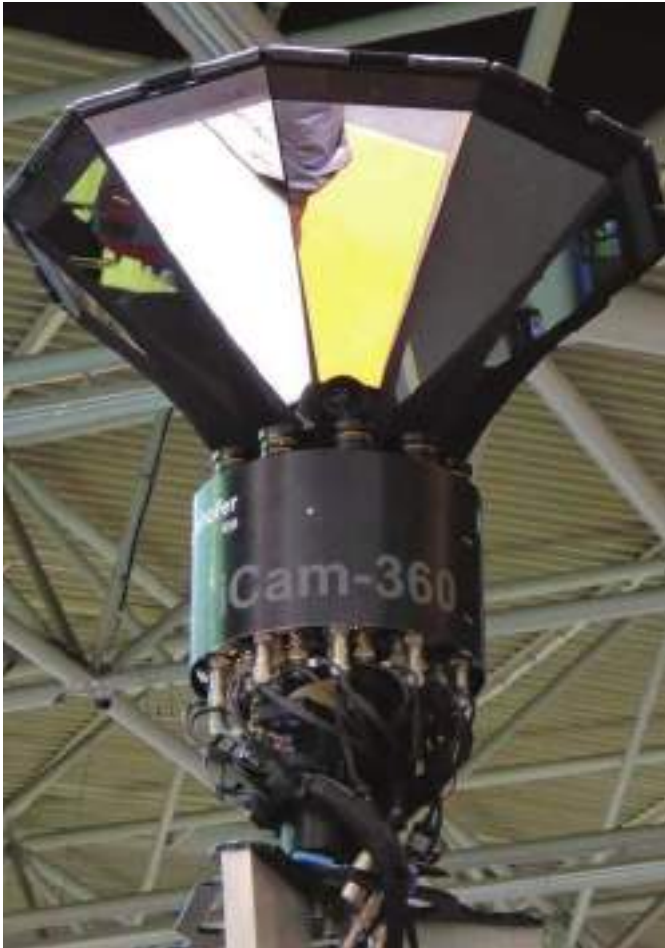
The Fraunhofer Institute for Telecommunications used 10 compact high-definition cameras facing upwards into a circular configuration of flat mirrors
